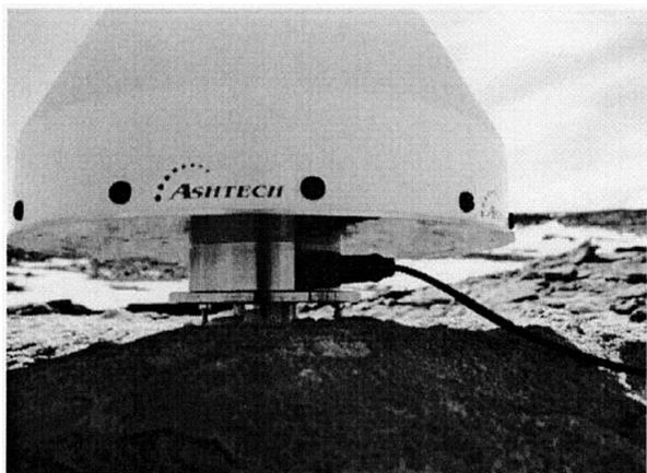
Fig. 4. Closeup of the GPS antenna mounting.
