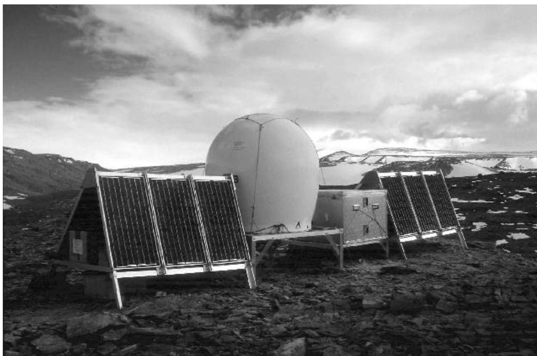
*Figure 6:* Equipment installed at Beaver Lake in February 2000. The white radome of the satellite phone can be seen between the solar panels, while all the electronics equipment is stored inside the silver box.
