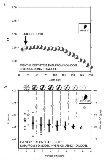
Figure 7. The results of synthetic test of: (a) depth sensitivity; (b) station selection sensitivity, for event #2 using synthetic data (no noise added). Synthetic data are produced using the 3-D model and inverted for the MT solution with synthetics based on 1-D model.
