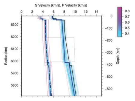
Figure 1. Results of a 20-parameter search by perturbing starting model–ak135 (black lines–*S*-wave velocity on the left, *P*-wave velocity on the right). Coloured lines show models tested and their average misfit (colour scale is shown on right; the lower the misfit the higher the fit). Thick blue lines indicate the best model found, which was only 1 per cent better than starting model.
