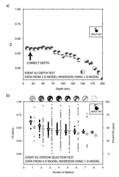
Figure 8. Same as Fig. 7, but for event #4: the results of synthetic test of: (a) depth sensitivity and (b) station selection sensitivity, using synthetic data (no noise added). Synthetic data are produced using the 3-D model and inverted for the MT solution with synthetics based on 1-D model.
