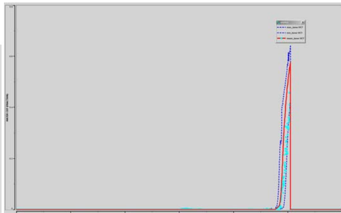
Figure 8: Comparison of Mean (red solid line), Maximum, and Minimum (blue dashed lines) Values of Simulation Results with Observation Data (cyan circles) of Water Cut in a Production Well
