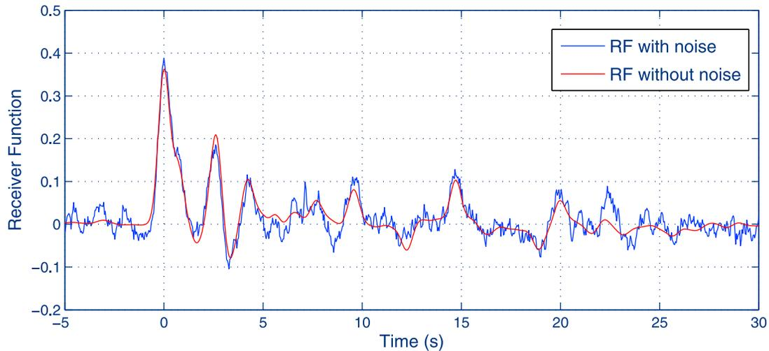
**Figure 2.** Simulated receiver function. Red: Synthetic data estimated from the true model in red in Figure 3. Blue: RF with added Gaussian random noise generated with an exponential correlation law (i.e.  $c_i = r^i$ ).
