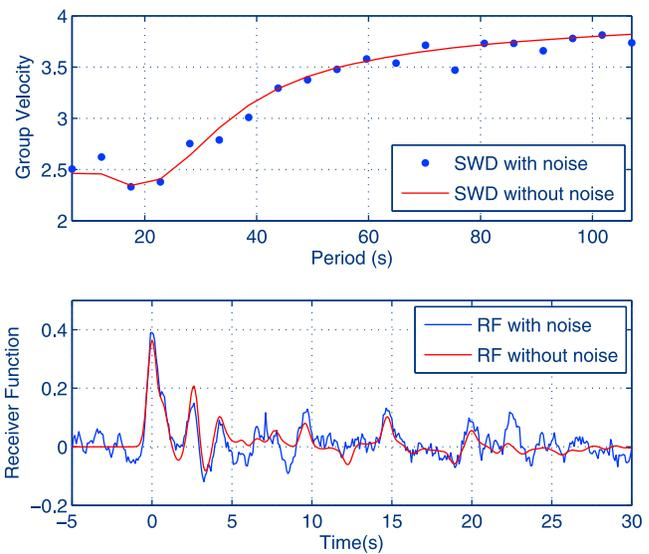
**Figure 9.** Simulated data with and without added noise for (top) SWD and (bottom) RF. In order to illustrate the benefits of a joint inversion, here the magnitude of noise added to the receiver function is larger than in sections 3.2 and 3.1.
