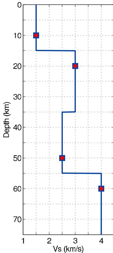
**Figure 1.** The model is parameterized with a variable number of Voronoi nuclei (red squares) which define the seismic structure (blue line). The vertical location of nuclei define the geometry of layers which Vs value is given by horizontal positioning of nuclei. Note that Voronoi nuclei are not necessary at the center of layers but rather boundaries are defined as equidistant to adjacent nuclei.
