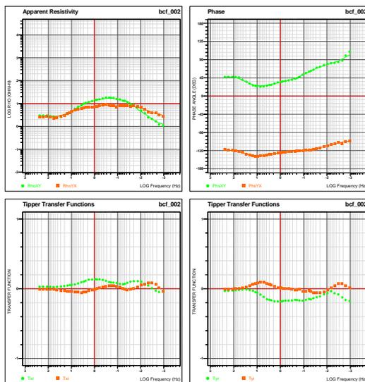
**Figure 2.** Example from site BC02 of apparent resistivity, phase (XY and YX) and tipper transfer function ( $T_{xy}$ ,  $T_{yx}$ ,  $T_{yz}$ ,  $T_{zy}$ ) sounding curves (from Stockill *et al.*, 2009).
