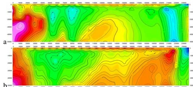
**Figure 4.** Pseudosections of the Bostick transform. (a) top, xy mode and (b) bottom, yx mode. The data represent the  $\log_{10}$  of the conductivity with blue low to red high. The width of the section is 240 km with south, left to north, right; the depth of the section is 50 km.
