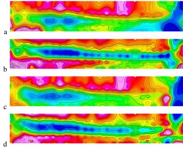
**Figure 3.** Pseudosections of apparent resistivity and phase. (a) top, xy apparent resistivity, (b) xy phase, (c) yx apparent resistivity, (d) yx phase. For (a) and (c) colours represent  $\log_{10}$  of conductivity; For (b) and (d) phase data are in degrees 0 to 90. Blue low to red high. The width of the section is 240 km, with south, left to north, right; the Y-axis represents frequency, with low, bottom to high, top.
