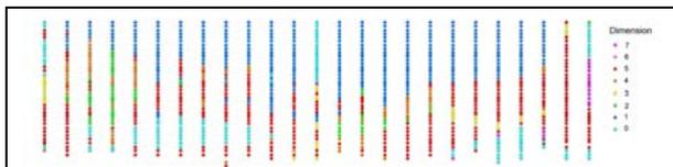
**Figure 5. Coloured circles representing dimensionality as determined from the WALDIM program. Horizontal axis represents site locations with south, left to north, right; the Y-axis represents frequency, with low, bottom to high, top.**
