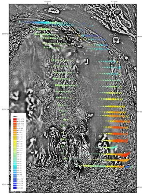
**Figure 7. Phase tensor ellipses, coloured by skew angle, for each site and period, with the shortest period centred on the site symbol. Background image is of the second vertical derivative of the total magnetic intensity, highlighting near-surface short-wavelengths of aeromagnetic data.**
