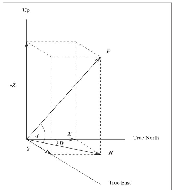
**Fig. 1. Components of Earth's magnetic field (total field  $F$ , horizontal component  $H$ , vertical component  $Z$ , north component  $X$ , east component  $Y$ , declination  $D$ , inclination  $I$ ). The orientation of the vertical component, which results in both  $Z$  and  $I$  having negative values, describes the southern-hemisphere magnetic field direction.**
