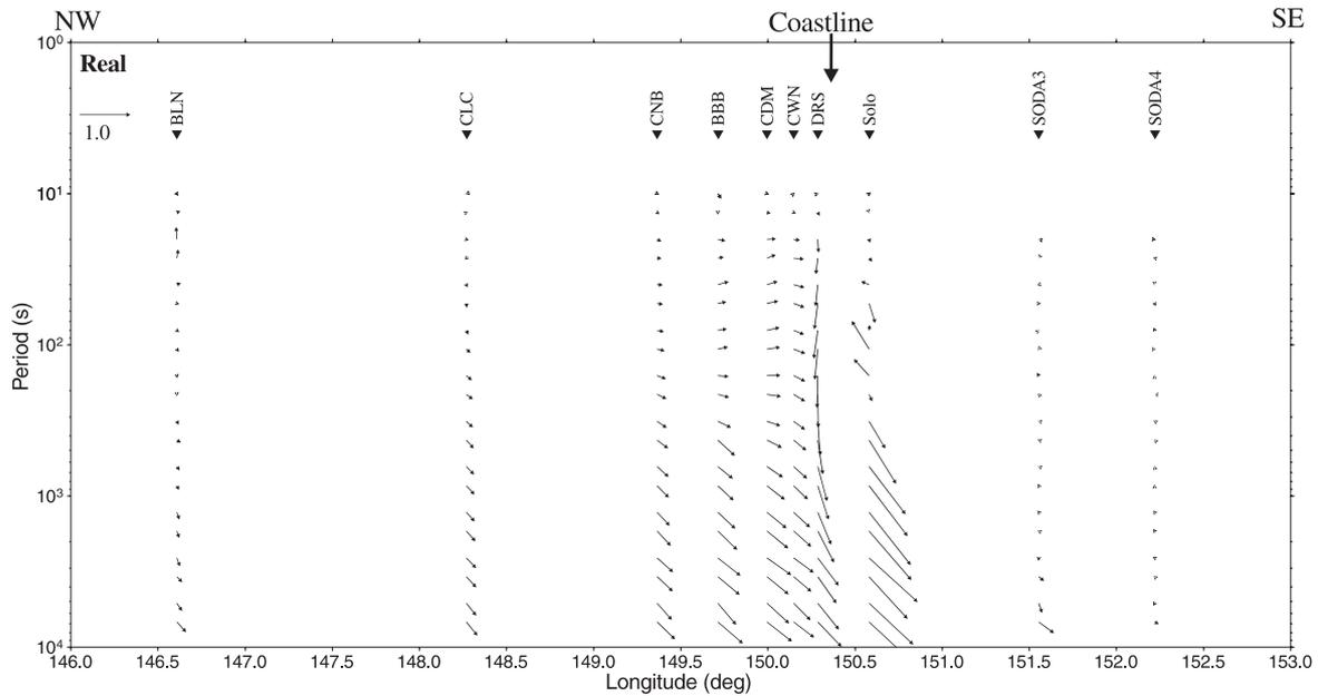
Fig. 6. Real induction arrows for the CICADA97 sites, derived using CNB as a reference site for horizontal variations. Data from days 274 to 276 were used for all stations, except BLN, where day 273 was used.
