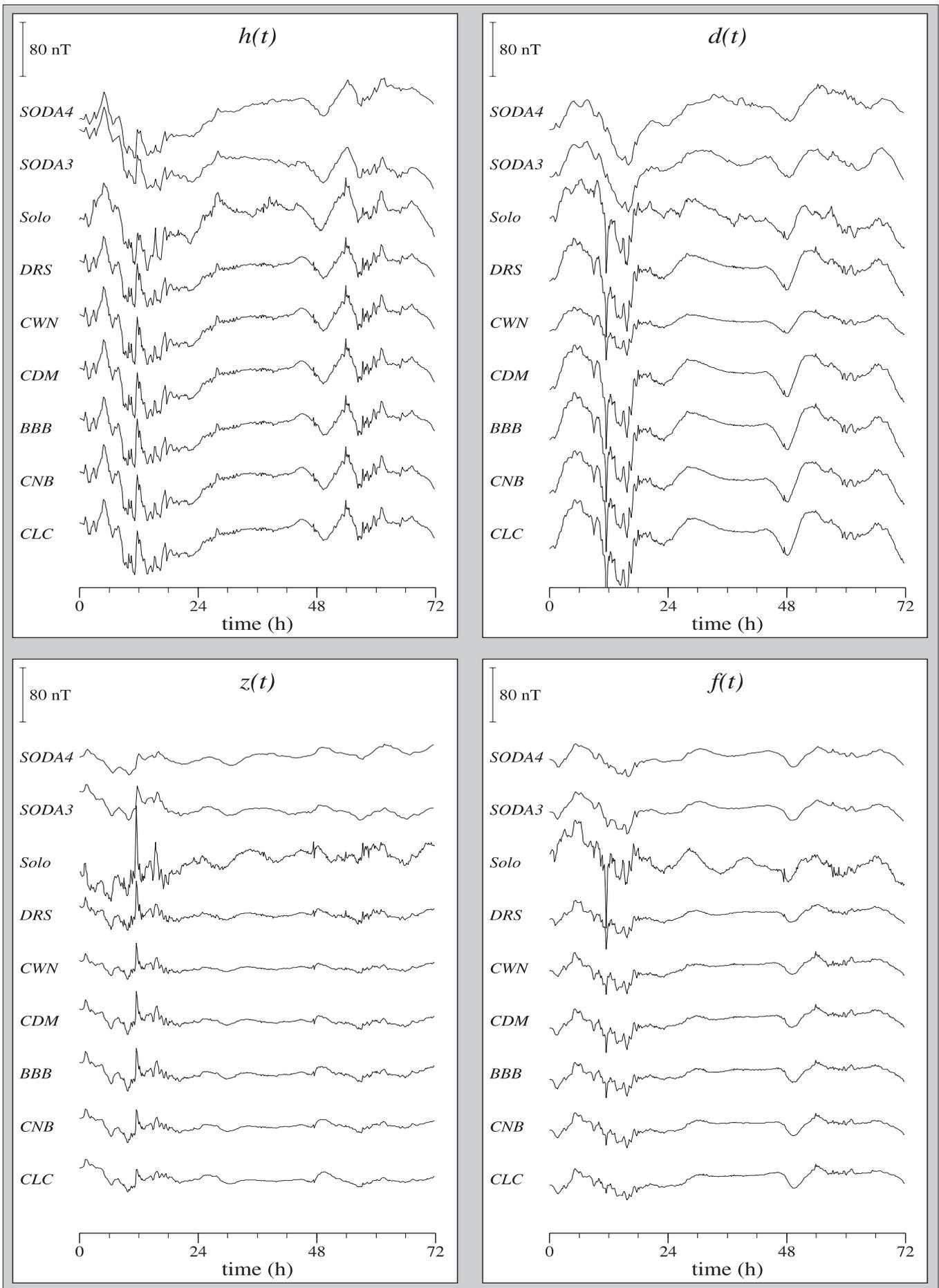
Fig. 3. Variations of the horizontal component, declination, vertical component and total-field ( $h(t)$ ,  $d(t)$ ,  $z(t)$  and  $f(t)$ , respectively) recorded at the CICADA97 sites. Data are for a 72 hr period consisting of day 274 to 276 (1 October to 3 October), 1997.
