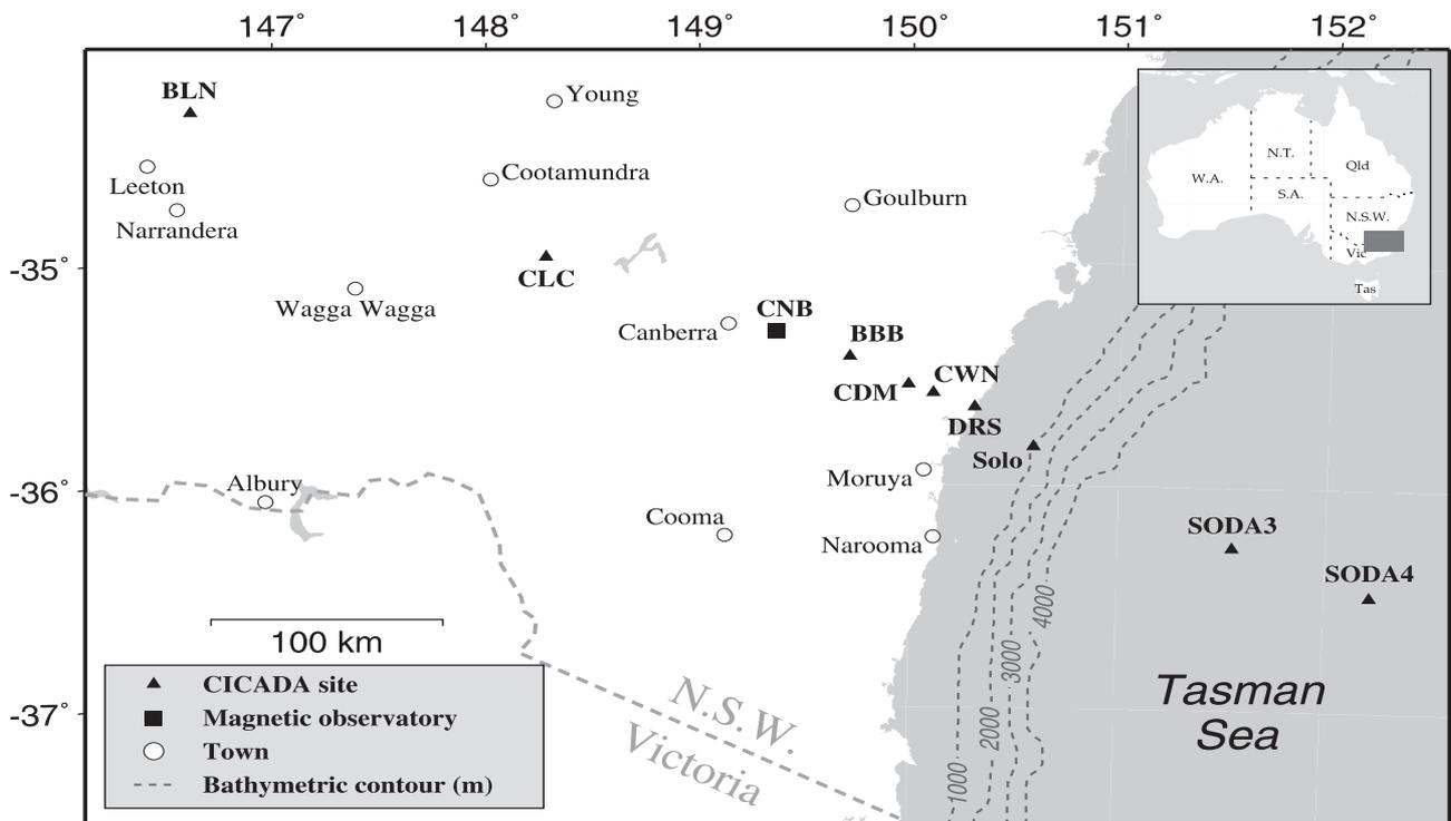
Fig. 2. Locations of CICADA97 stations used to investigate the total-field implications of the geomagnetic coast effect. CNB is the Canberra magnetic observatory operated by AGSO. The ‘D’ of DRS marks the position of Batemans Bay, referred to in the text.
