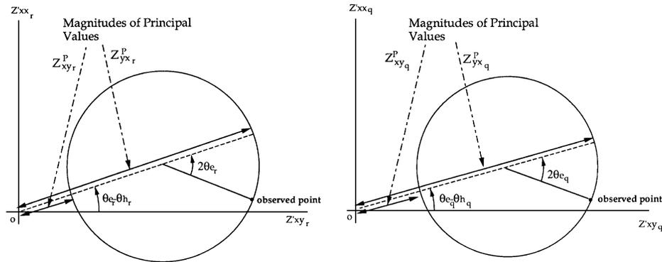
FIG. 8. Diagram showing the decomposition parameters  $\theta_{er}$ ,  $\theta_{hr}$ ,  $\theta_{eq}$ , and  $\theta_{hq}$  and the magnitudes of the principal values  $Z_{xy_r}^P$ ,  $Z_{yx_r}^P$ ,  $Z_{xy_q}^P$ , and  $Z_{yx_q}^P$  on a type 1 diagram. This diagram also shows how a circle that (due to error) encloses the origin will be invalid for the determination of a minor principal value.
