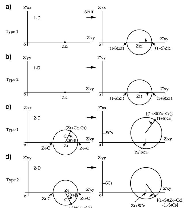
FIG. 5. Effects of a splitting operator on 1-D cases (a and b) and 2-D cases (c and d) for both type 1 and type 2 diagrams. The left-hand and right-hand columns are before and after application of the splitting operator. Here  $c$  and  $s$  denote  $\cos \beta'$  and  $\sin \beta'$ , respectively.
