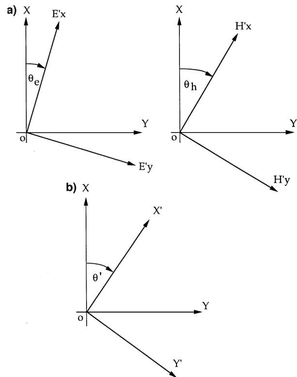
FIG. 1. Geometry for rotation of measuring axes. (a) The case for the basic theorem, where the  $E$  axes are rotated angle  $\theta_e$ , and the  $H$  axes are rotated angle  $\theta_h$ . (b) The common case, where the measuring axes  $XOY$  are rotated angle  $\theta'$  clockwise to  $X'OY'$  for both  $E$  and  $H$  fields.
