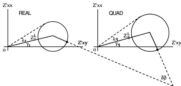
FIG. 4. A pair of real and quadrature circles for a tensor, showing the set of invariants  $Z^L_r$ ,  $\lambda_r$ ,  $\gamma_r$ ,  $Z^L_q$ ,  $\lambda_q$ ,  $\gamma_q$ , and  $\delta\beta$  by which the complete tensor may be specified.
