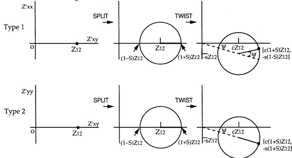
FIG. 7. Mohr diagrams for paths 1 and 2. Here  $c$  and  $s$  denote  $\cos \psi$  and  $\sin \psi$ , where  $\psi$  is the twist.
