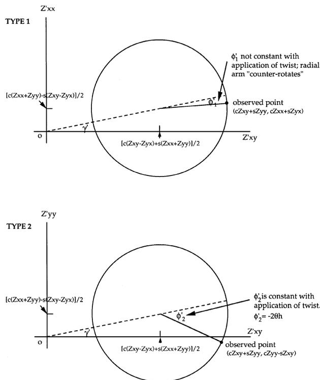
FIG. 6. The effects of a twist operator on diagrams of type 1 and type 2 (as described in the section on twist). Here *c* and *s* denote  $\cos \psi$  and  $\sin \psi$ , where  $\psi$  is the additional twist applied to the general cases of Figure 2.
