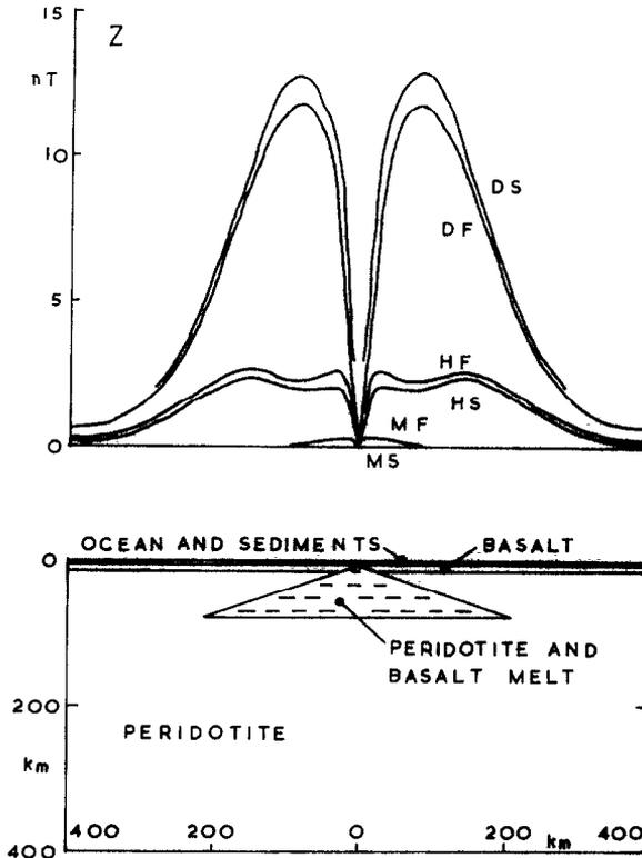
Fig. 2. Electrical conductivity model for a mid-ocean ridge and its electromagnetic response, from Duba and Lilley (1972).  $Z$  is the amplitude of the vertical component of magnetic field fluctuation due to the ridge structure.  $D$ ,  $H$  and  $M$  stand for fluctuations of period 1 day, 1 h and 5 min, respectively.  $F$  and  $S$  stand for measurements at the sea floor and sea surface, respectively. The inducing field is horizontal across the ridge and of amplitude 50 nT.
