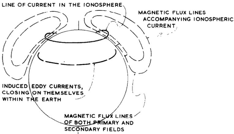
Fig. 1. Sketch of the process of natural electromagnetic induction in the earth. All the magnetic fields and electric currents shown vary with time.
