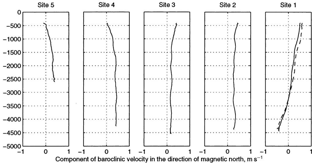
**Figure 10.** Downcast data from sites 1 to 5, median-filtered, corrected for winch speed, and reduced to give profiles of the component of baroclinic velocity in the direction of magnetic north. Each such profile needs a zero shift to convert it to actual velocity, and such zero shifts are shown carried out in Fig. 12. The lower half of the profiles for site 1 are considered to be influenced by seafloor magnetization effects and should be ignored from an oceanographic point of view.
