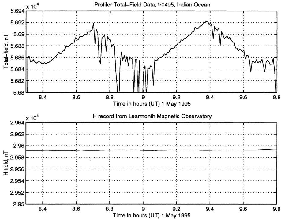
**Figure 5.** Profiler (total-field) and Learmonth Observatory (H-component) data, May 1995, Indian Ocean, site 4. The casts are to near-bottom, in water 1800 m deep. The major sections of the record evident are, in order: downcast, upcast, downcast, upcast. Note wind speed varies at the start and finish of each cast. As for the upcast in Fig. 4, the noise spikes recorded during the upcasts are attributed to degraded magnetometer performance, possibly caused by vibration.
