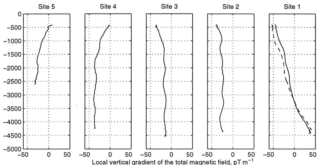
**Figure 9.** Downcast data from sites 1 to 5, median-filtered, corrected for wind speed, and reduced to give profiles of the vertical gradient of the total magnetic field. The ordinate of the plots is depth in m. The dashed line at site 1 indicates a second cast there, approximately 2.5 hr after the first cast.
