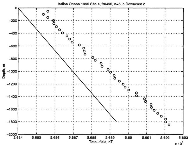
**Figure 6.** Downcast data from Indian Ocean site 4, median-filtered, and corrected for wind speed. Also shown is a line with the gradient predicted for the site by the IGRF. The actual surface value predicted by the IGRF is 56924 nT, which can be seen to be some 80 nT greater than observed. The magnetic effects of the ship in the upper 300 m of the cast are evident.
